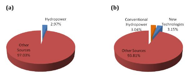
Comparison of (a) the region's current hydropower energy capacity, with (b) the potential capacity including the proposed hydrokinetic and conventional hydropower developments.
